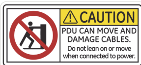
Figure 3-9 Warning label located on PDU
